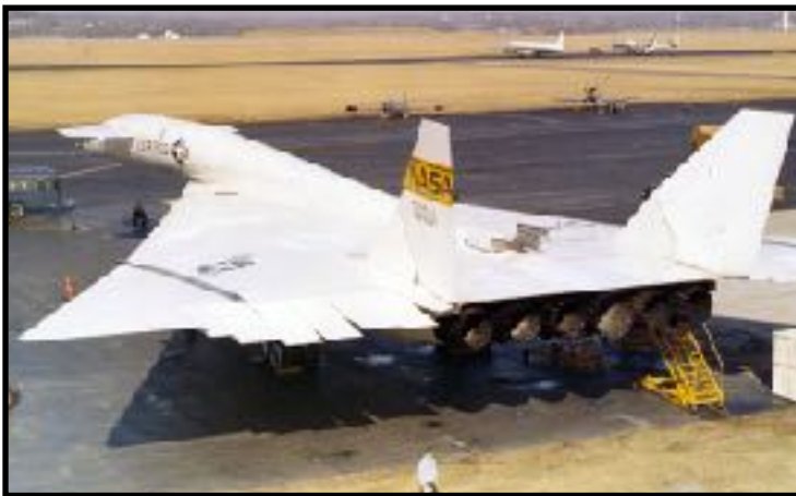
Figure 7 Elevon Surfaces on Trailing Edge
